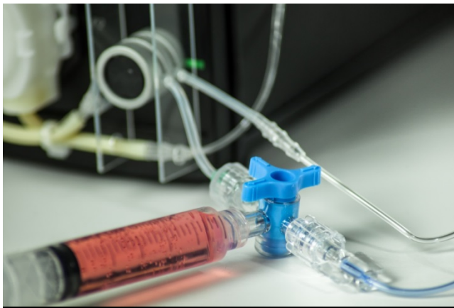
Figure 76: Connecting the external sample
