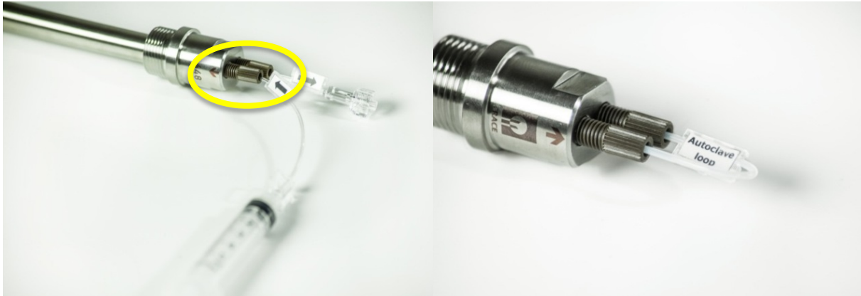
Figure 55: Filling the dialysis probe with buffer solution Figure 56: Sealing the probe prior to sterilization (autoclave loop)
