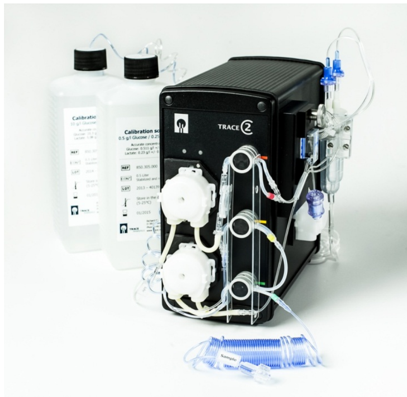
Figure 12: Ready-for-use installation of The device (filtration mode)
