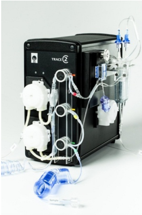
Figure 27: View of fully-equipped front panel for the „Filtration“ operating mode
