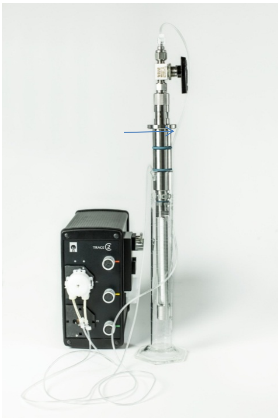
Figure 60: Setup and connection of the hydrophilizing set
