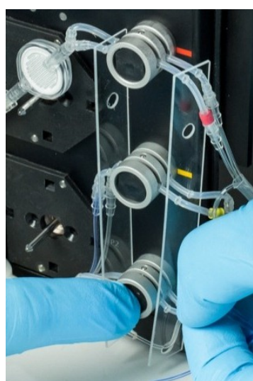
Figure 28: Manually switching the valve to insert the rear tube securely.
