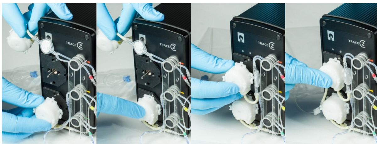
Figure 31: Attaching lower pump cassette P2 and upper pump cassette P1
