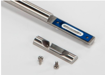
Figure 43: Inserting a new membrane
