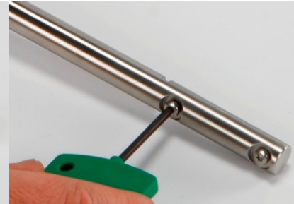
Figure 45: Tightening the 2 screws
