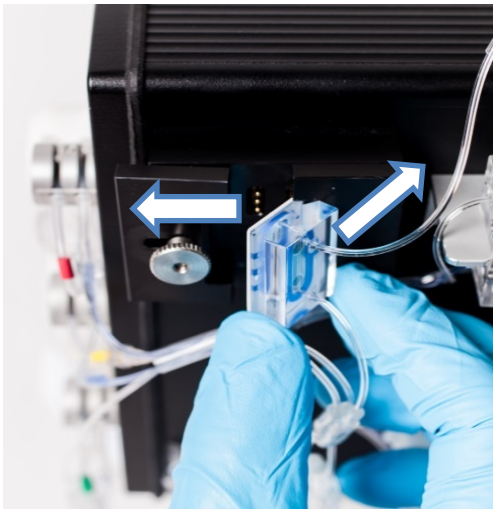
Figure 33: Inserting the measurement cell into the device
