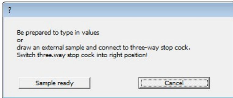
Figure 67: Prompt for sampling and connection to the three-way stopcock
