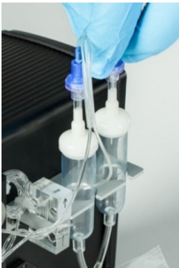
Figure 36: Inserting the drip counters into the holder
