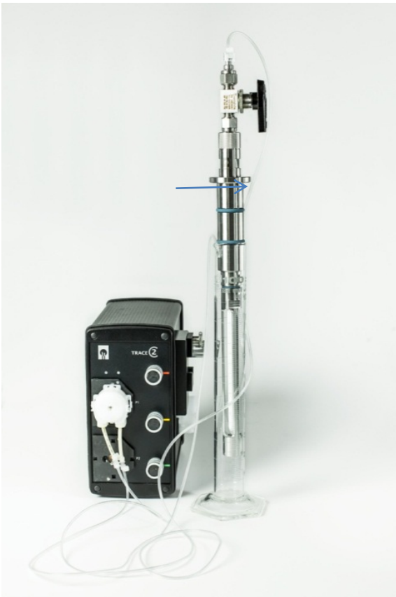
Figure 53: Setup and connection of the hydrophilizing set
