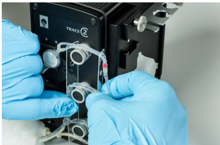
Figure 26: Position of the valve tubes on the device
