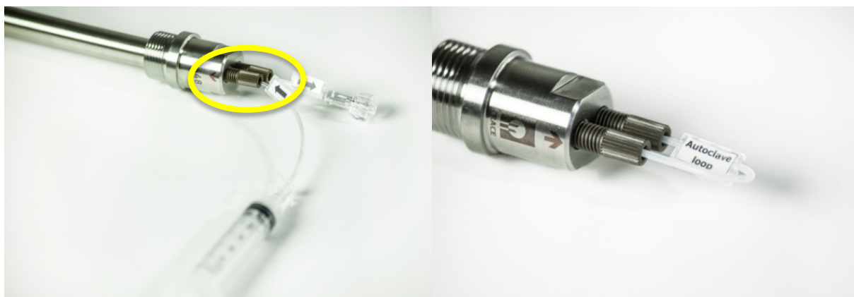
Figure 48: Filling the dialysis probe with buffer solution Figure 49: Sealing the probe prior to sterilization (autoclave loop)
