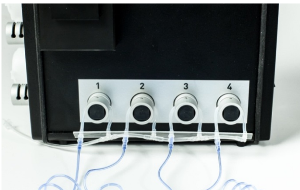
Figure 37: Assembling of the selection valves at the MultiTRACE
