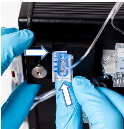
Figure 34: Fastening the measurement cell to the device
