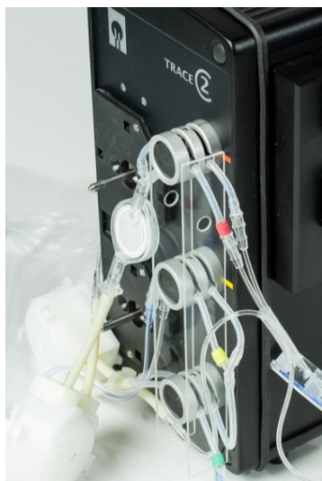
Figure 29: Securing the valve tubes by pushing together the guide plates
