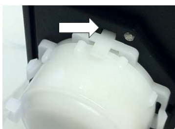
Figure 30: Proper placement of the pump cassette (fastening stud locked in place)
